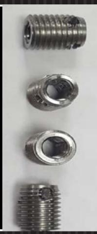
**Hex Drive Inserts** Currently available with an M5 internal thread with an M8 x 1mm (fine pitch) external thread. This insert offers a 4mm hex drive which runs through the full length, meaning this insert is a popular choice as it can easily be inserted with nothing more than a hex drive key or allen key.
