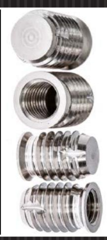
These inserts offer standard metric internal threads with 30 degree inclusive form coarse pitch self-tapping external threads. We would recommend blind self-tapping inserts for use in applications where fluid ingression along the internal thread could be an issue.
