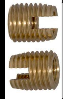
Our 'off the shelf' INS300 inserts have standard through-tapped metric internal threads. These type of inserts generally have a fine pitch metric external thread, designed to be self-cutting and is not intended for insertion into pre-tapped holes.
